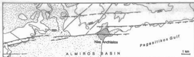
Fig. 3: Sketch map of the Nea Anchialos Fault. Topographic contours every 200 m. Dotted areas are Pleistocene-Holocene deposits. See Fig. 1 for location.
