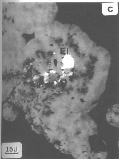
Fig. 2a-d: a. Sub-rhombic adularia crystals, ore stage. (crossed polars) b. Electrum aggregates or crystals (type 1) included and/or intersticed between ore-stage fine-grained quartz. c. Electrum (type 2) and fine-grained native gold (type 3) included in iron oxides. d. Intergrowth of colloform iron oxides, native gold (type 3) and halogens of silver (todyrite, cerargyrite).
