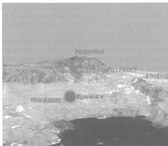
Figure 2a) Perspective view (towards northeast at 35° above the horizon) of western Attica, Greece. The image was constructed using computer vision techniques, TM imagery (741 RGB) and a 20-m DEM. Dark gray line is the trace of the Fili normal fault that moved during the 7/9/1999 earthquake. Vertical exaggeration x 3. 2b) Shaded relief image of a Digital Elevation model of the seisoseismal area simulating orientation of topography with respect to an illumination source (SE-140; zenith angle of 75 degrees). Light gray line is the Thriassion normal fault; gray line is the Fili normal fault. Crosses are aftershock epicentres; Gray circle is the relocated NOAGI epicentre of the main shock of Sept. 7, 1999. Map shows also the distribution of rock falls (white circles). Roman capital letters indicate the earthquake intensity.
