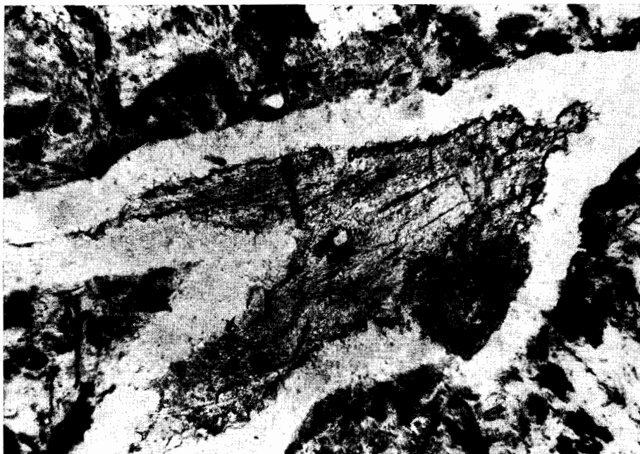
Fig. 7. Calcite 3 generation separated in the core of quartz vein. Plane pol. light.
