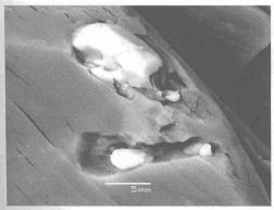
Figure 13 - Celestite crystals in vugs on gypsum
