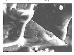
Figure 10 - Dissolution patterns of gypsum
