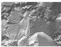
Figure 6 - Interlocking crystals of gypsum
