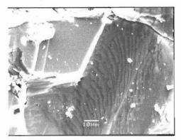
Figure 5 - Dissolution patterns of gypsum
