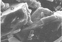
Figure 8 - Bassanite small crystals generating from gypsum
