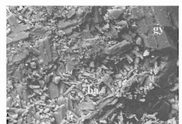
Figure 7 - Bassanite (small crystals) on gypsum
