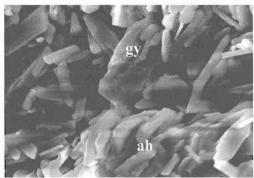
Figure 12 - Anhydrite small crystals aud gypsum (center)
