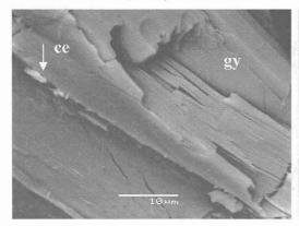
Figure 19 - Celestite (ce) developed ou boundaries of deformed gypsum (gy)
