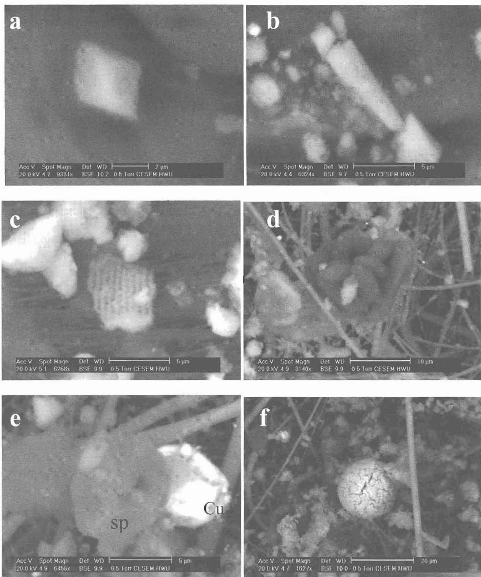
Figure 4 - Classification of airborne particles according to their origin: a) a geogenic rhombohedral calcite, b) an elongated quartz crystal, c) a fragment of diatom frustules belonging to Centrophycae class (biogenic), d) fungal spores (biogenic), e) a spore/pollen (biogenic) [sp] and a Cu-rich partiele (anthropogenic) [Cu], f) a Fe-rich, fly ash plerosphere (anthropogenic)
