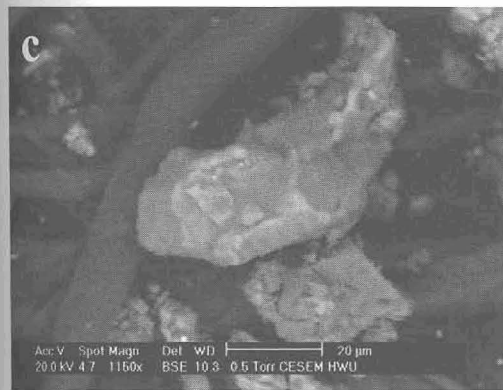
Figure 5 - ESEM images and EDX spectra of airborne particles of different composition: a) a feldspar crystal [(K,Na,Ca)AlSi 3 O 8 ], b) a clay or mica flake, c) a calcium carbonate [CaCO 3 , calcite] particle
