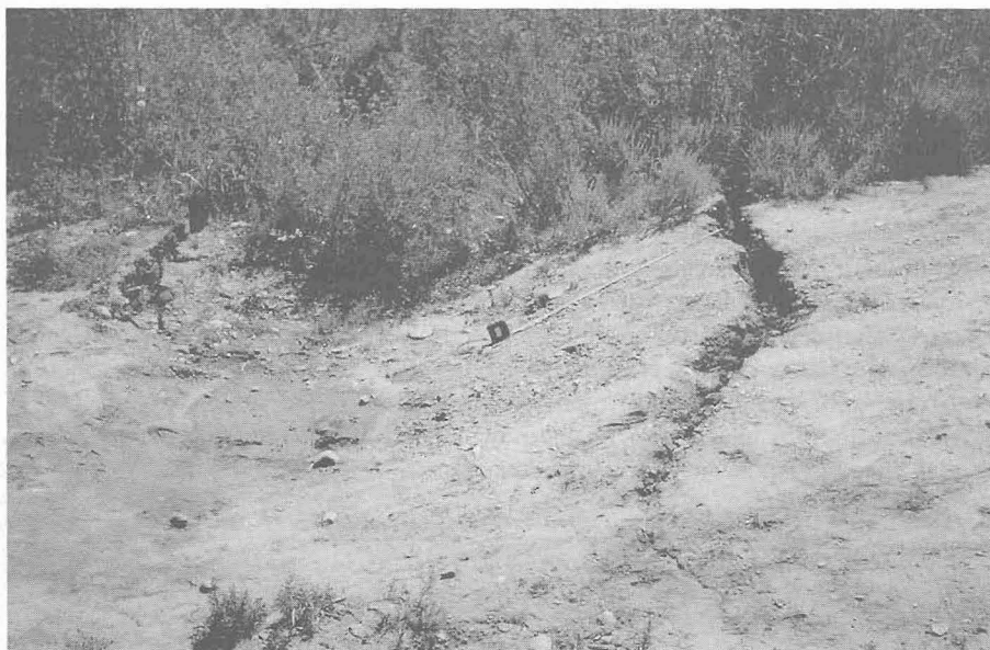
Figure 1 – The suffosion-subsidence processes above the underground sewer systems
