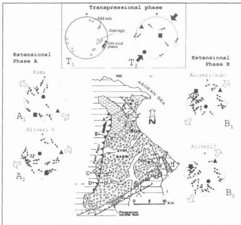
Figure 3. Geological map of the Kymi basin and equal-area, lower hemisphere stereonet with fault planes shown as poles and striae as arrows onto the poles. In stereonet the filled circle indicates the position of s_1 stress axes, the rectangular the position of s_2 and the triangle the position of s_3 .
