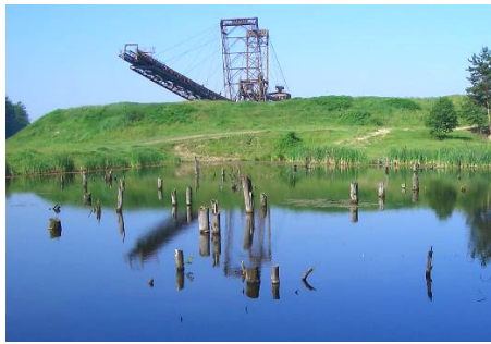
Photo 7: Lake formed through the blocking of the Amaradia river by the waste dump placed in the floodplain, at Poiana Seciurle
