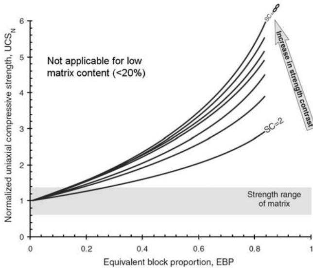
**Fig. 6:** Relationships between equivalent block portion (EBP) and UCS of Ankara agglomerate, with lines of different strength contrast (ratios) between andesite blocks and tuff matrix (after Sonmez et al., 2006).
