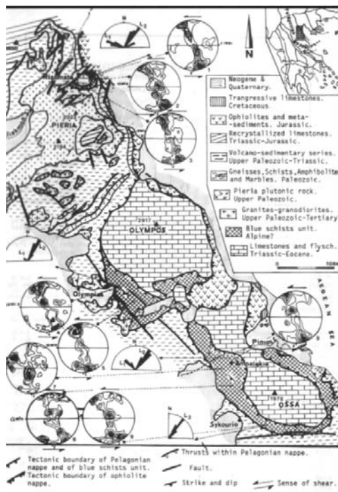
Fig. 4: Geological map of the Olympos Ossa window (from Kiliias et al., 1991). The rock falls area is located in Ambelakia – Ossa unit.
