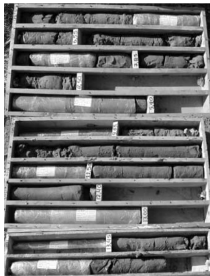
Fig. 3: Test drilling core samples taken from the broader area of Nafplio (Pantelias, 2009).
