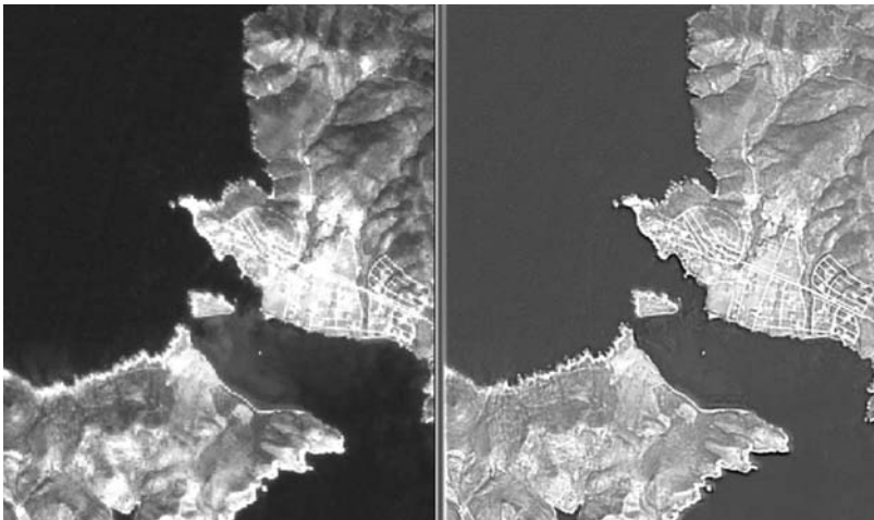
Fig. 2: (left): The Gram-Schmidt fused image at 1/25.000 scale. A RGB combination of specific bands (2203, 844, 487 nm) is presented; (right): The same RGB combination of the HPF fused image.
