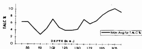
Fig. 4: Moving average data for Talc % (Table 3) versus Depth, based on 18 data points and a moving period of 2. It is evident that after 150 m and with increasing depth there is a strong tendency of increase the Talc %.
