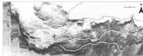
Fig. 9. Side scan sonar sonograph showing: (a) the paleoshoreline of 11-14m, (b) the paleoshoreline of 22-24m and (c) the Dokos wreck location.
