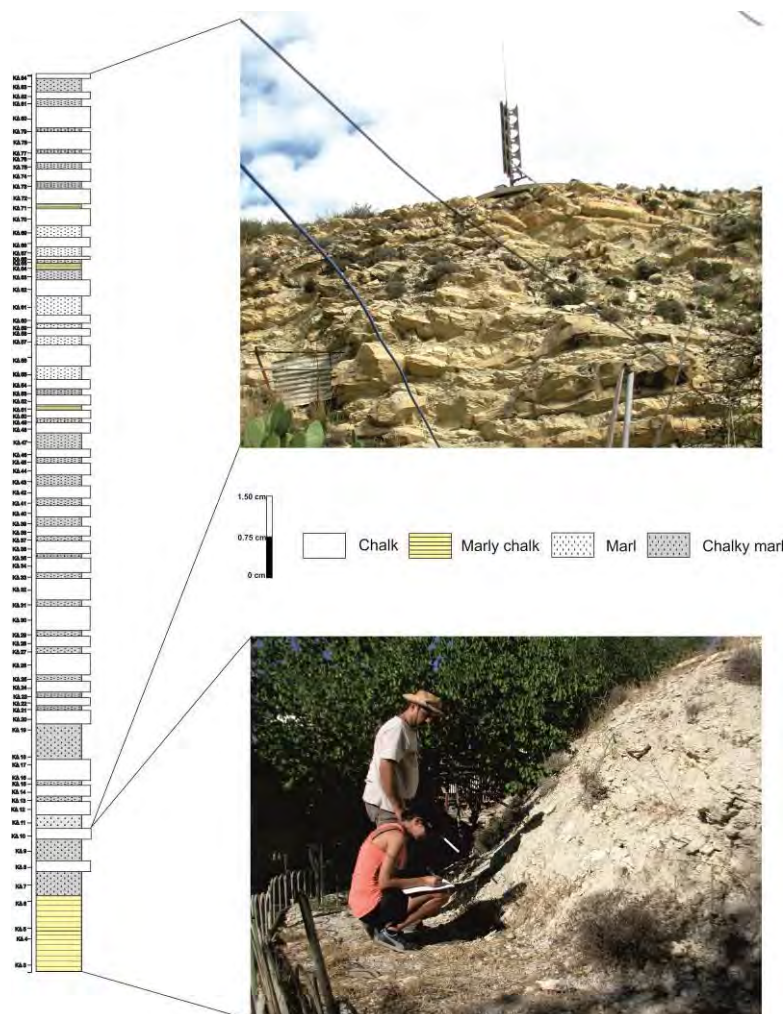
Figure 2 - Detailed lithostratigraphy of Kotaphi Hill section and sample location.
