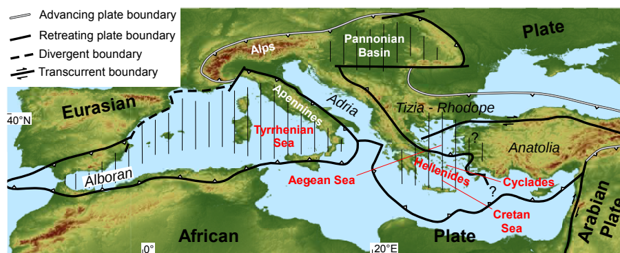
Figure 1 - Highly simplified tectonic map of the Mediterranean plate boundary zone showing retreating, advancing, and major transcurrent plate boundaries (barbs on overriding plate). Shown are the three major plates (Eurasia, Africa, Arabia) and, schematically, microplates between the three major plates; these microplates are currently forming (e.g., Anatolia) or have been amalgamated to Eurasia in the past (e.g., Adria). Vertical lines indicate highly extended regions above retreating plate boundaries (after Ring et al., 2010).
