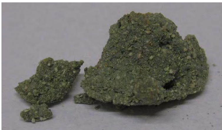
Figure 4 - Odourless and cohesive zeosludge, dried at room temperature for 24 hours.
