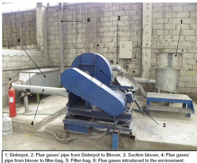
Figure 1 - Pilot-scale sintering installation.
