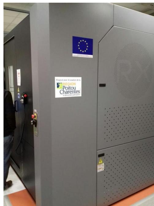
Figure 5. On the left, the scanning chamber with the detector monitor, the scanning skull *P. anubis* C2 and the X-ray source. On the right, the microCT scan EasyTom XL Duo at Centre 113 de Microtomographie (IC2MP, iPHEP, Université de Poitiers).
