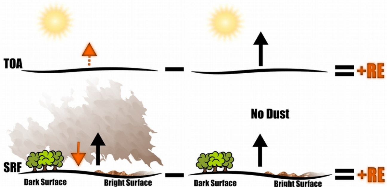
Figure 1.11. Illustration of the dust longwave radiative effect (RE) at the surface (SRF) and at the top of the atmosphere (TOA). Left and right panel depicts a dust loaded and a dust free atmosphere respectively. Vectors indicate the downward and upward radiation. The orange colored vectors correspond to a positive radiative effect of dust particles.
