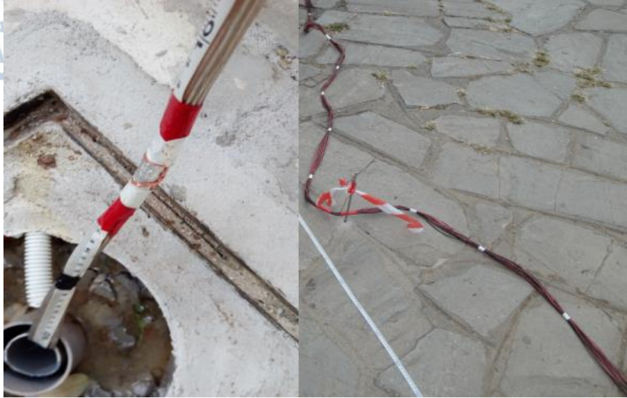
Figure 5.3: The borehole and surface electrodes, used for the field measurements.
