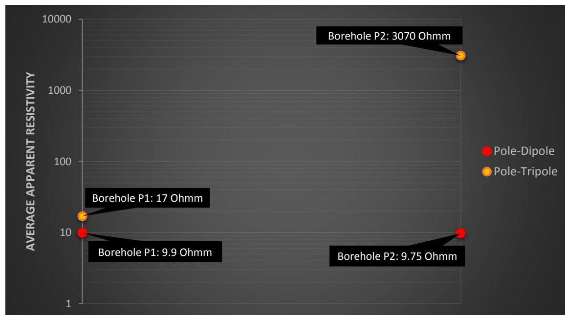
Figure 5.7: Plot of the average apparent resistivity for the pole-dipole and pole-tripole arrays, separately, for each borehole.
