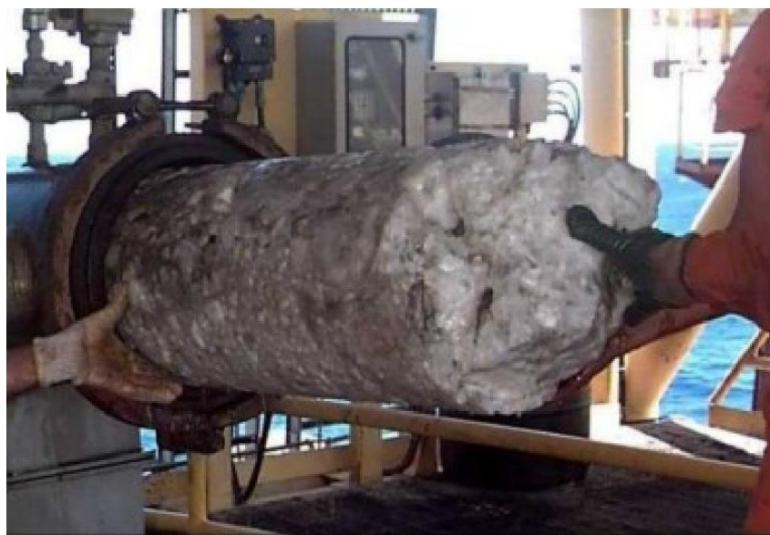
Fig. 2.2.11 Hydrate Plug Formed in a Subsea Hydrocarbon Pipeline (adopted from https://www.uio.no/studier/emner/matnat/math/MEK4450/h11/undervisningsmateriale/modul-5/MEK4450_FlowAssurance_pensum-2.pdf )
