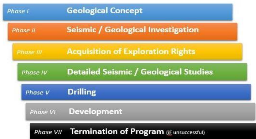
Fig. 4.1 Typical exploration-exploitation stages (adopted from https://www.glossary.oilfield.slb.com )
