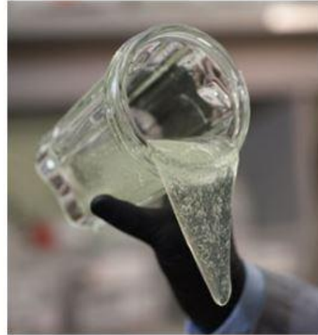
Fig. 4.10 Sand proppant and chemical additive for hydraulic fracturing (Adopted from https://geology.com )
