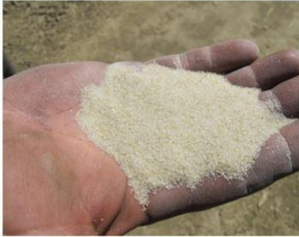
Fig. 4.10 Sand proppant and chemical additive for hydraulic fracturing (Adopted from https://geology.com )
