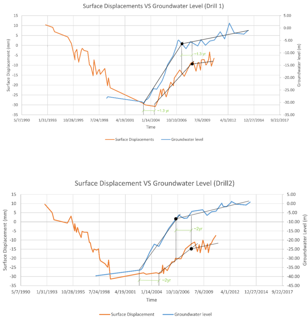
Figure 4.10 Upper panel: Graph comparing the ground water level variations at Drill 1 with the surface deformation time series at a nearby data point produced by the SAR analysis. Lower panel: Graph comparing the ground water level variations at Drill 2 with the surface deformation time series at a nearby data point produced by the SAR analysis (Svigkas et al. 2016).
