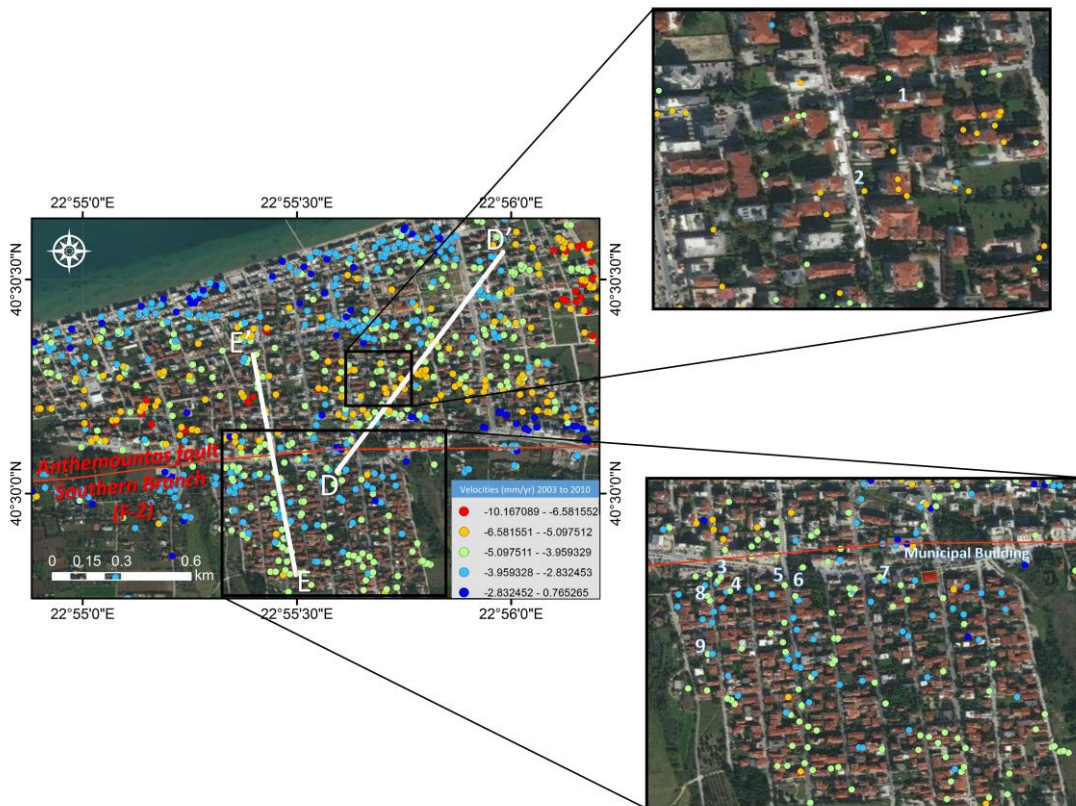
Figure 4.23 Close-up of the area of Perea (rectangle 3 in Fig. 4.11 and rectangle 3 in Fig. 4.16b) showing the displacement of the second monitoring decade (ENVISAT). Velocities in the area show that some locations are stable and others are deforming (with maximum velocity -10 mm/yr). The red line is the southern branch of Anthemountas fault (F-2 in Fig. 4.16b). The white lines in the map are the velocity profiles (E'-E, D'-D) presented in Figure 4.18. Numbers in the two smaller inset maps to the right, are showing in detail the surface velocities occurring at the area together with numbering that represents the failures detected during the field investigation. A picture for each failure number is shown in Figure 4.24.
