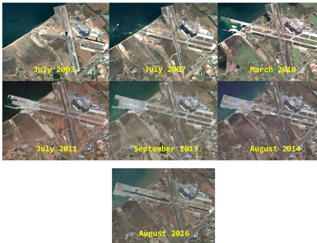
Figure 4.21 Evolution of the construction phases of the extension of runway 10-28 to the northwest. The existence of water and the frequent changes of the land pattern have created a loss of coherence on the part of the runway that is extending over the sea (images from google Earth).
