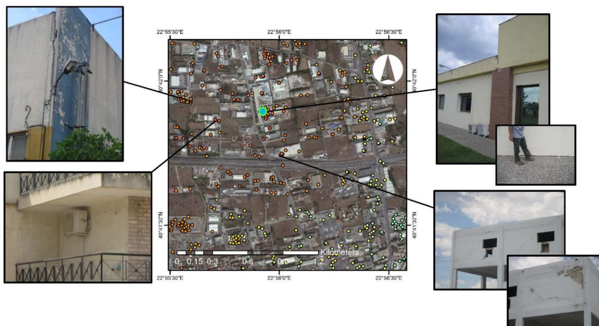
Figure 4.34 Map showing the correlation of the time-series measurements of the first decade (subsidence) with failures detected in the field (left and right). The light blue-light green dot is a point whose time-series is presented in Figure 4.35 (Svigkas et al. 2017).
