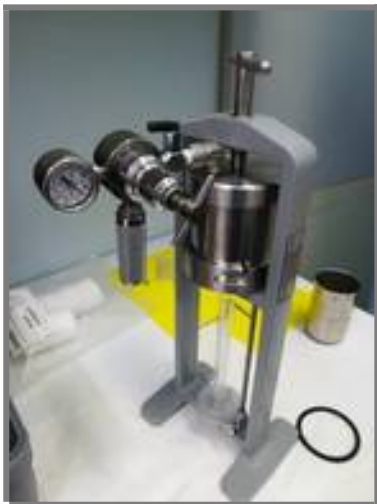
Figure 21. Fann LP/LT filter press Basic Assembly Specifications.
