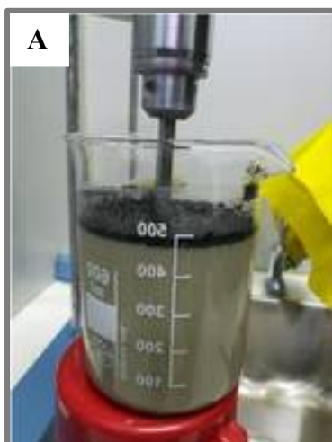
insoluble coal sample in drilling fluid, showing no significant dissolution.
