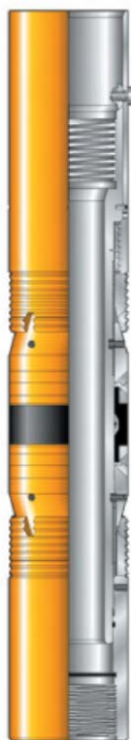
Fig.3.34 Permanent sealbore packer (Lake, 2007).
