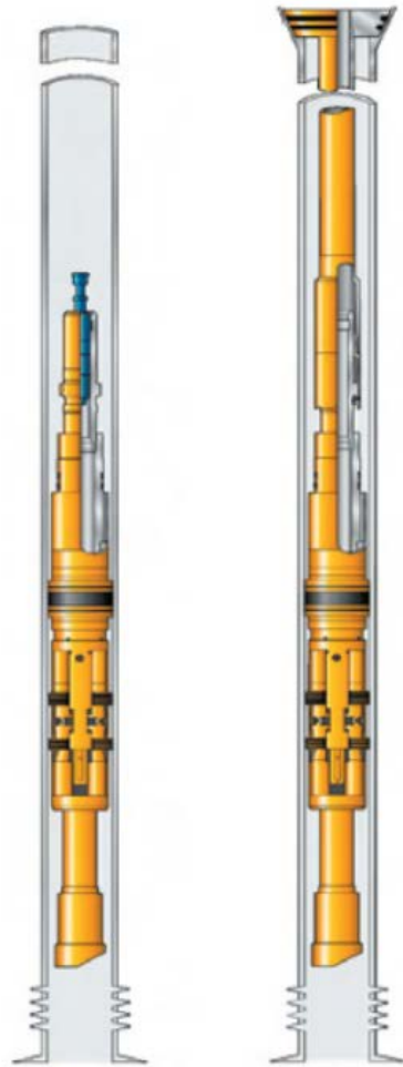
Fig.3.30 A set with plug in place (left) and with tubing connected and plug retrieved (right) of Wireline-set tubing retrievable packer (Lake, 2007).
