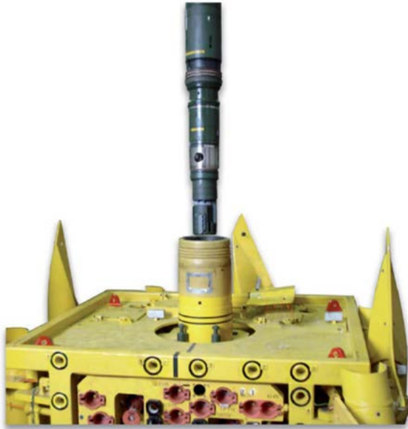
Fig.3.43 Horizontal subsea tree with tubing hanger (Bellarby, 2009).
