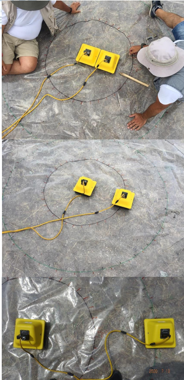
Figure 92: Data acquisition in the area of interest for the endfire antenna orientation and for the circles of r=0.23\text{m} (top), r=0.5\text{m} (middle), r=1\text{m} (bottom).
