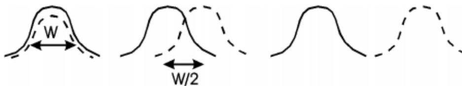
Figure 10: Considering the pulse envelope, two events could be well resolved if they are separated in time by W/2 (Annan, 2003)
