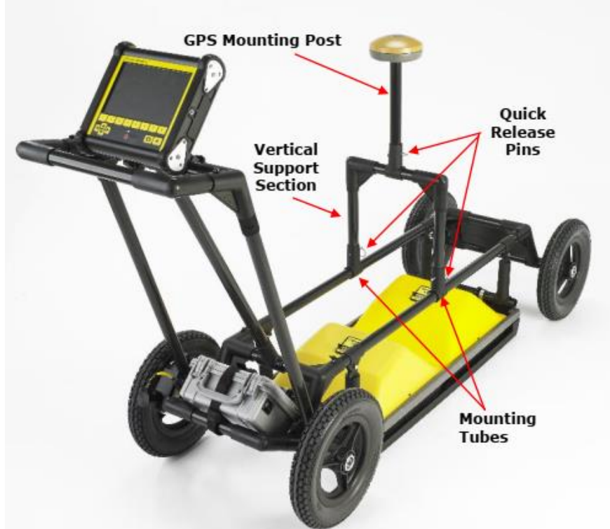
Figure 90: The SmartCart GPR system from Sensors & Software (top left corner and bottom) and the SmartCart GPR system configured for operation with 500MHz transducers for the GPR grid data acquisition in the area of interest (top right corner).
