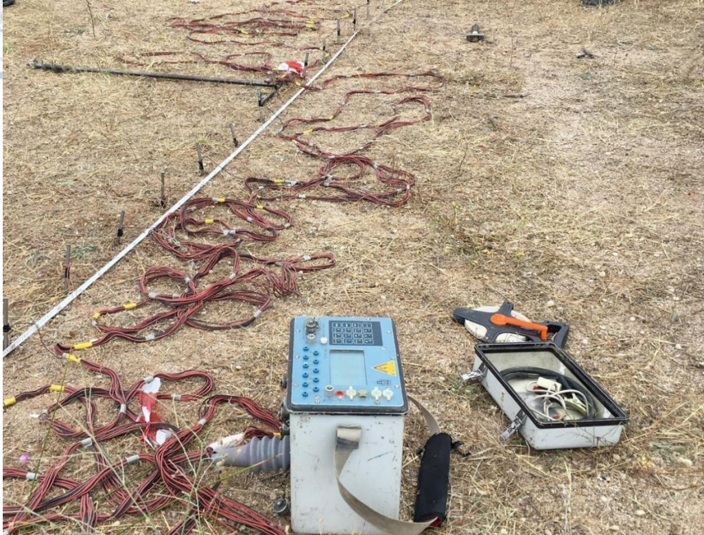
Figure 94: Data acquisition for the ERT measurements in the area of interest. The electrodes are at a dipole-dipole arrangement and they are connected to the SyscalPro of Iris Instruments.
