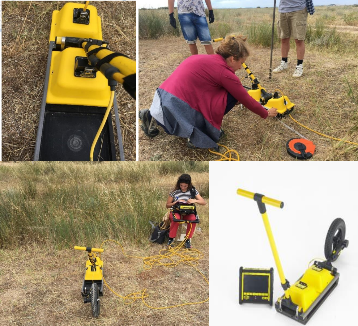
Figure 91: Data acquisition for the WARR measurements with the pulseEKKO 500 SmartTow GPR system. Example for the broadside antenna orientation (top left corner) with antenna spacing equal to 0.275m (top right corner).
