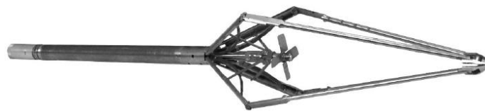
Figure 64: PFCS Full-bore flowmeter with built in X-Y caliper ( Courtesy: Schlumberger ).
