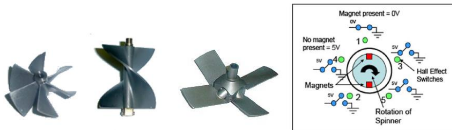
Figure 62: Various types of spinners – Schematic of the Hall effect ( Courtesy: Sondex ).
