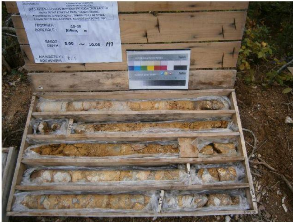
Borehole (Γεώτρηση) ΔΟ-30 – Depth (Βάθος) 5.00~10.00m
