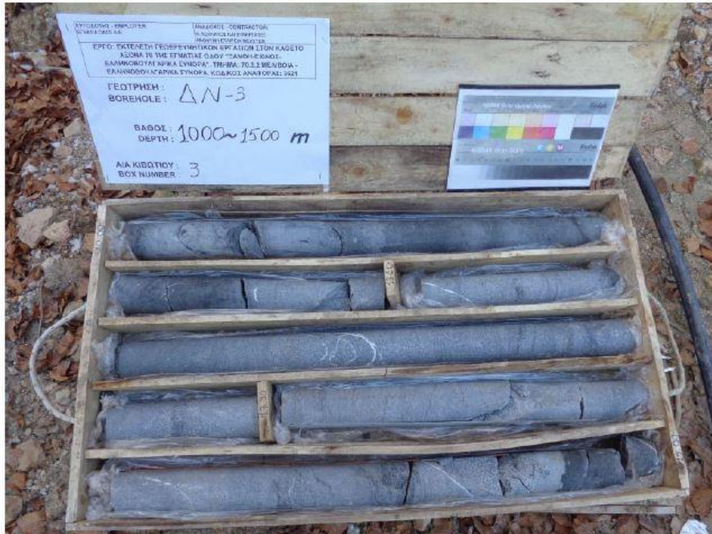
Borehole (Γεώτρηση) ΔN-3 – Depth (Βάθος) 10.00~15.00m
