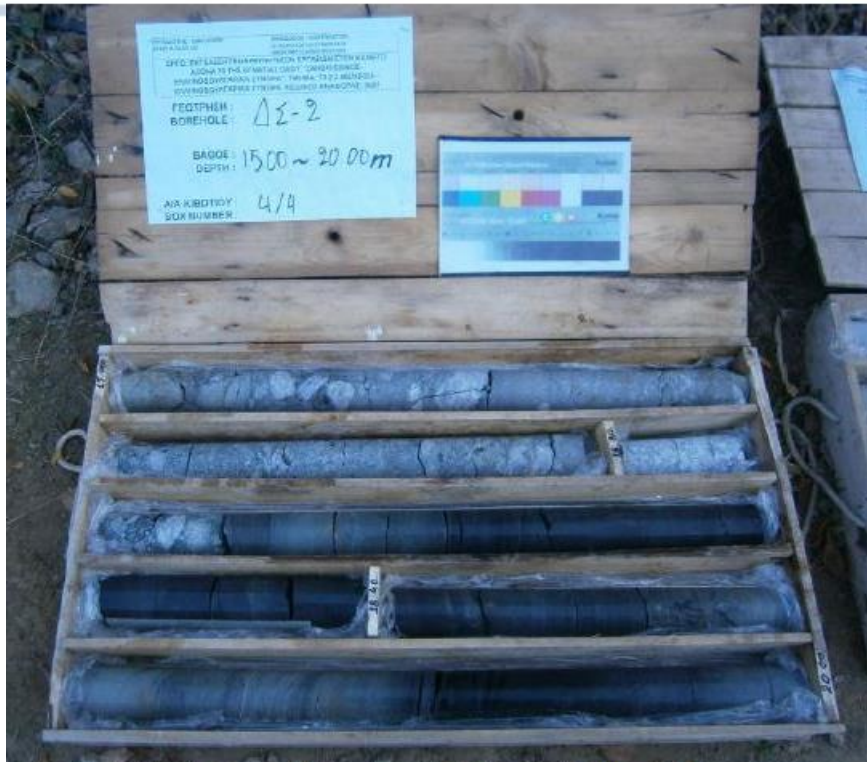
Borehole (Γεώτρηση) ΔΣ-2 – Depth (Βάθος) 15.00~20.00m
