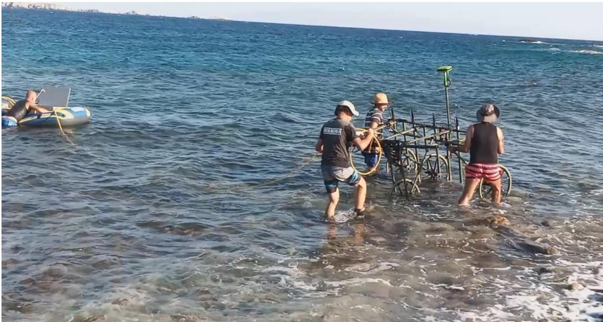
Figure 2.2: Sensorik & Systemtechnologie (SENSYS) MX Compact Survey System mounted on a plastic frame during the survey in the very shallow part of an archaeological site.
