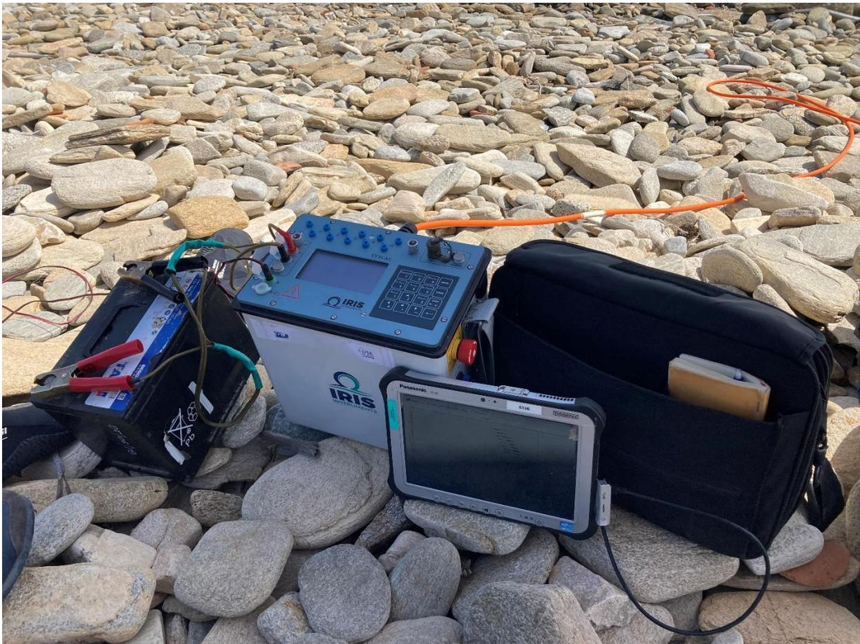
**Figure 2.7:** The Syscal Pro Switch resistivity tomography system along with an external battery and a toughpad
