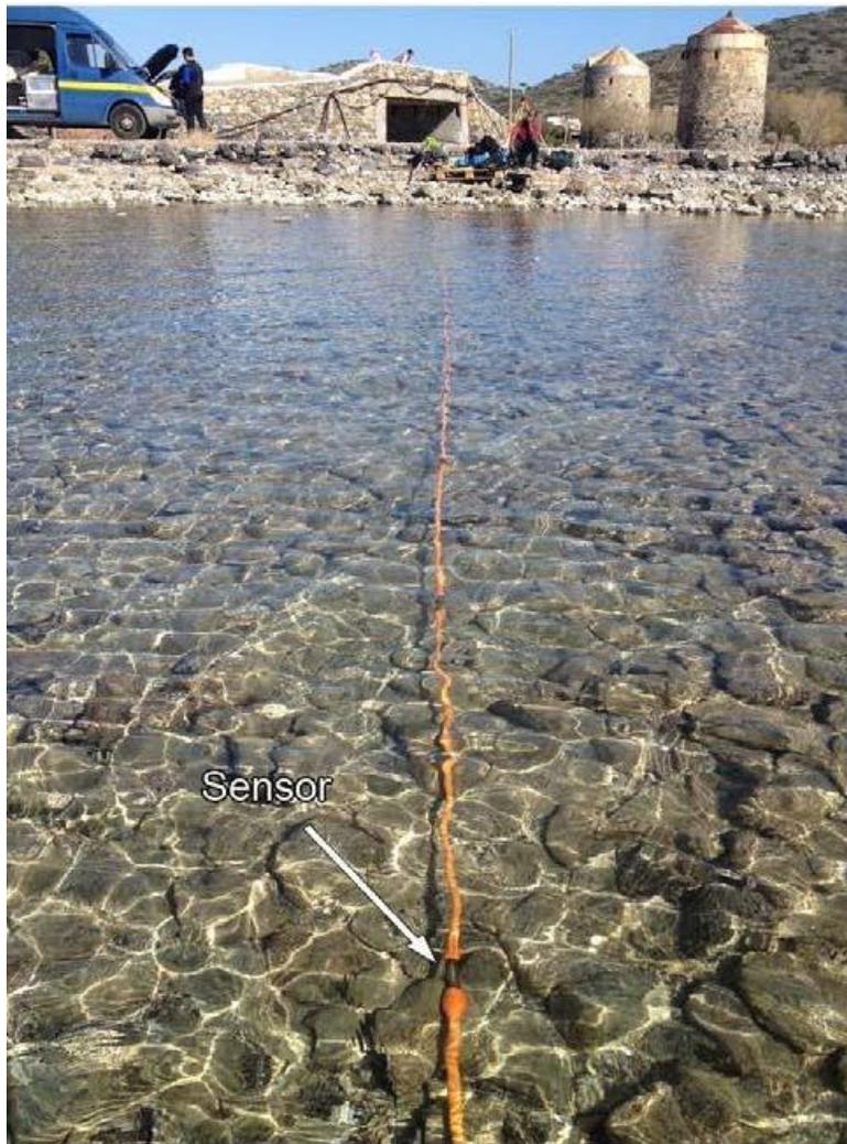
Figure 2.9: View of the submerged cable with the stainless-steel electrodes attached on the sea bottom to complete the Static ERT Survey
