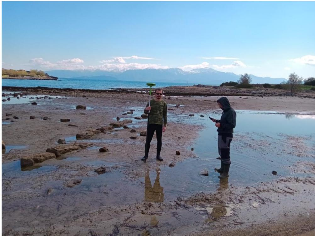
Figure 2.6: GNSS unit mounted on a pole and used as a rover for the shallow bathymetric survey
