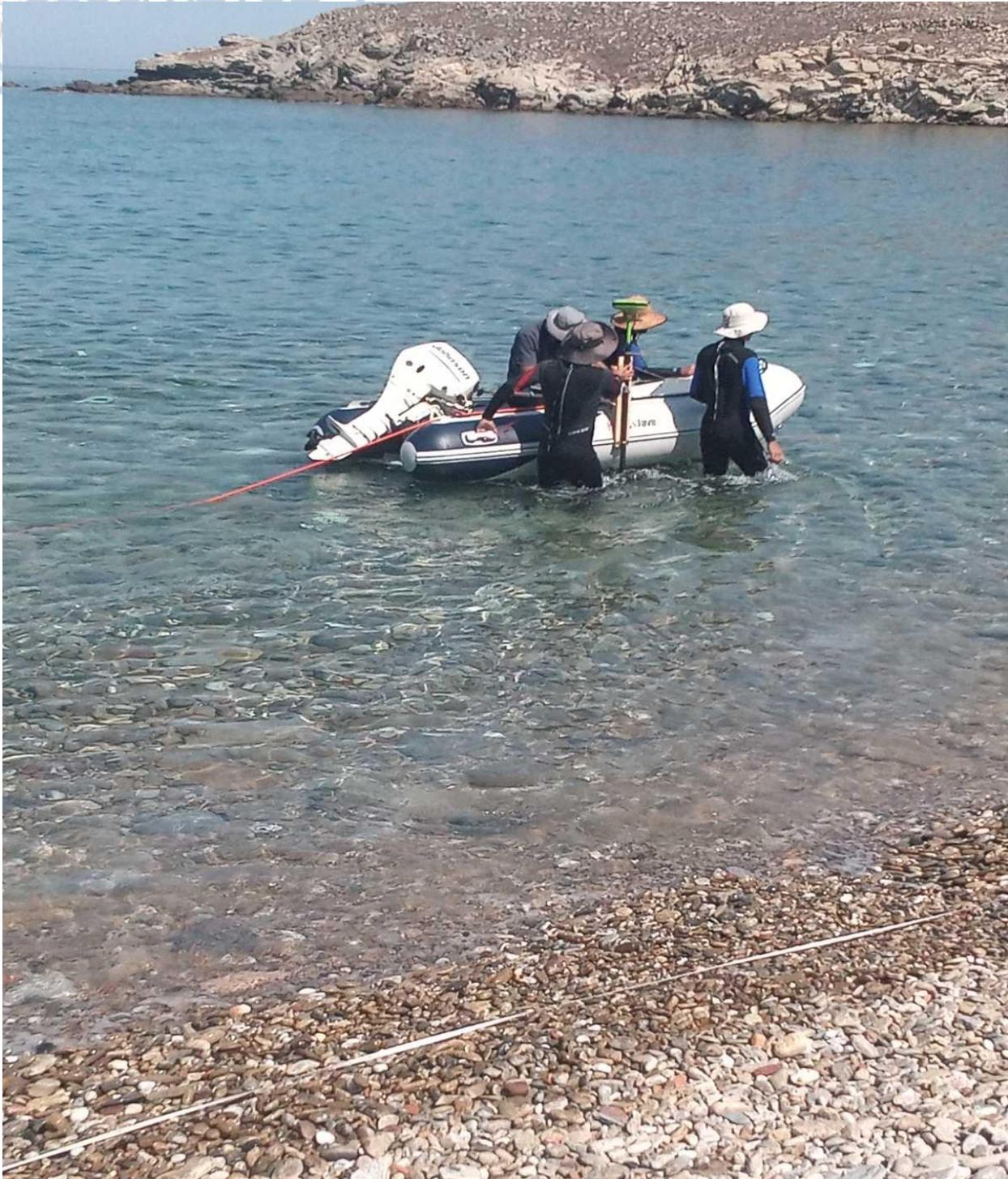
Figure 2.8: In situ ERT survey with dynamic lines to cover the ultra shallow part of the site in Skardhanas.
