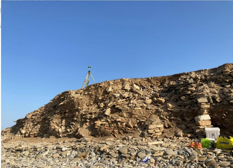
Figure 2.5: Base GNSS Unit which is constantly communicating with a rover unit.
