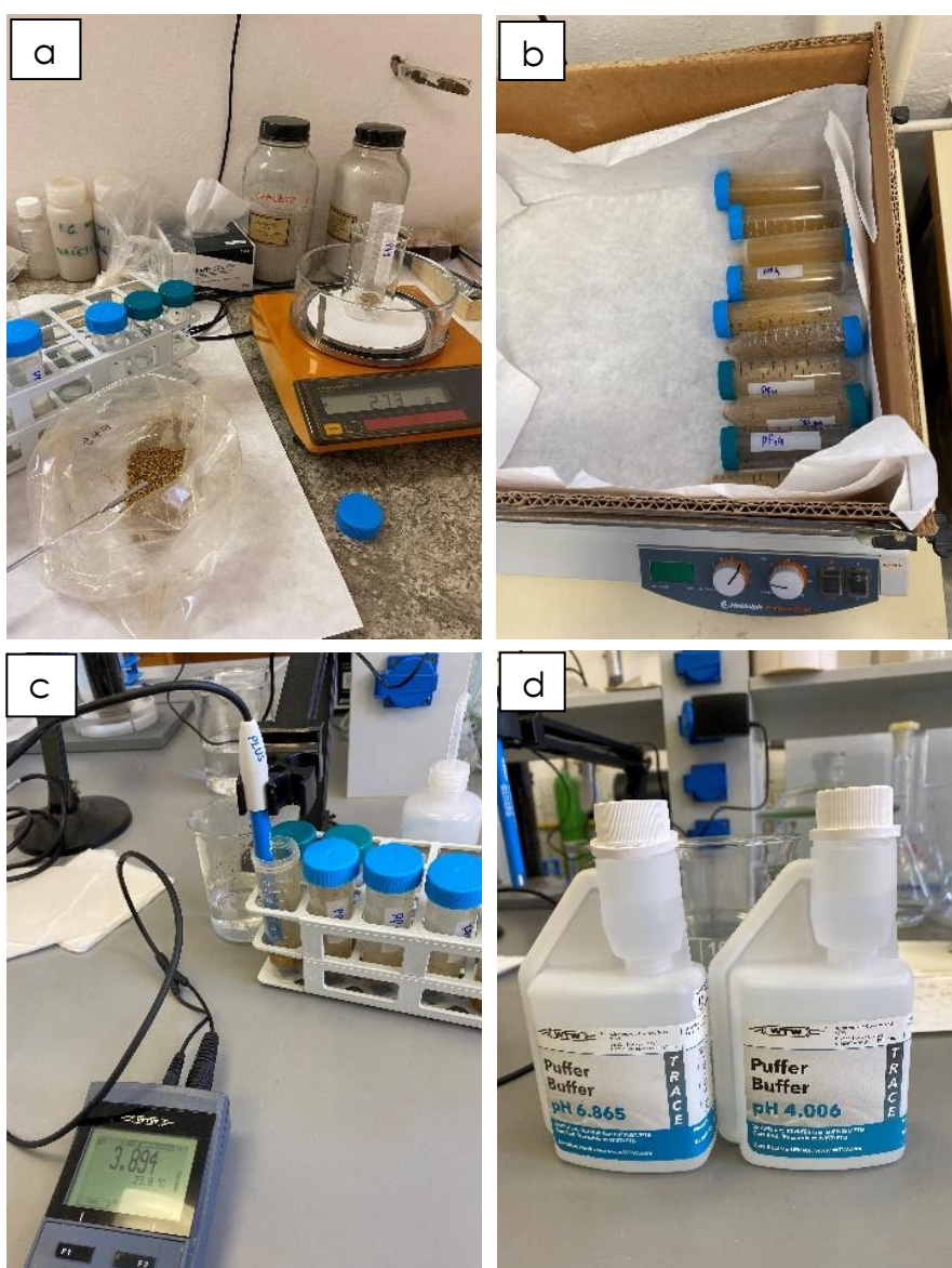
Fig. 9. Equipment and procedures of the pH measurement: a. weight of dried samples, b. horizontal shaker, c. WTW multimeter and combined electrode, d. buffers
