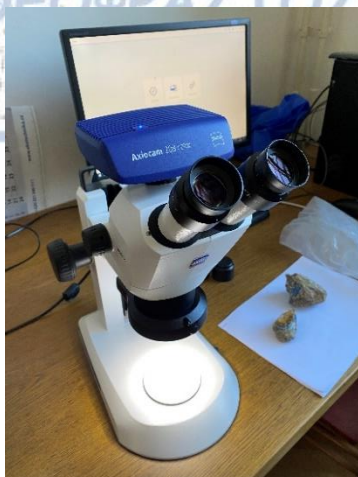
Fig. 17. Zeiss Stereo Microscope used for the detection of the secondary phases in samples A2, B4, S in the form of polished sections.
