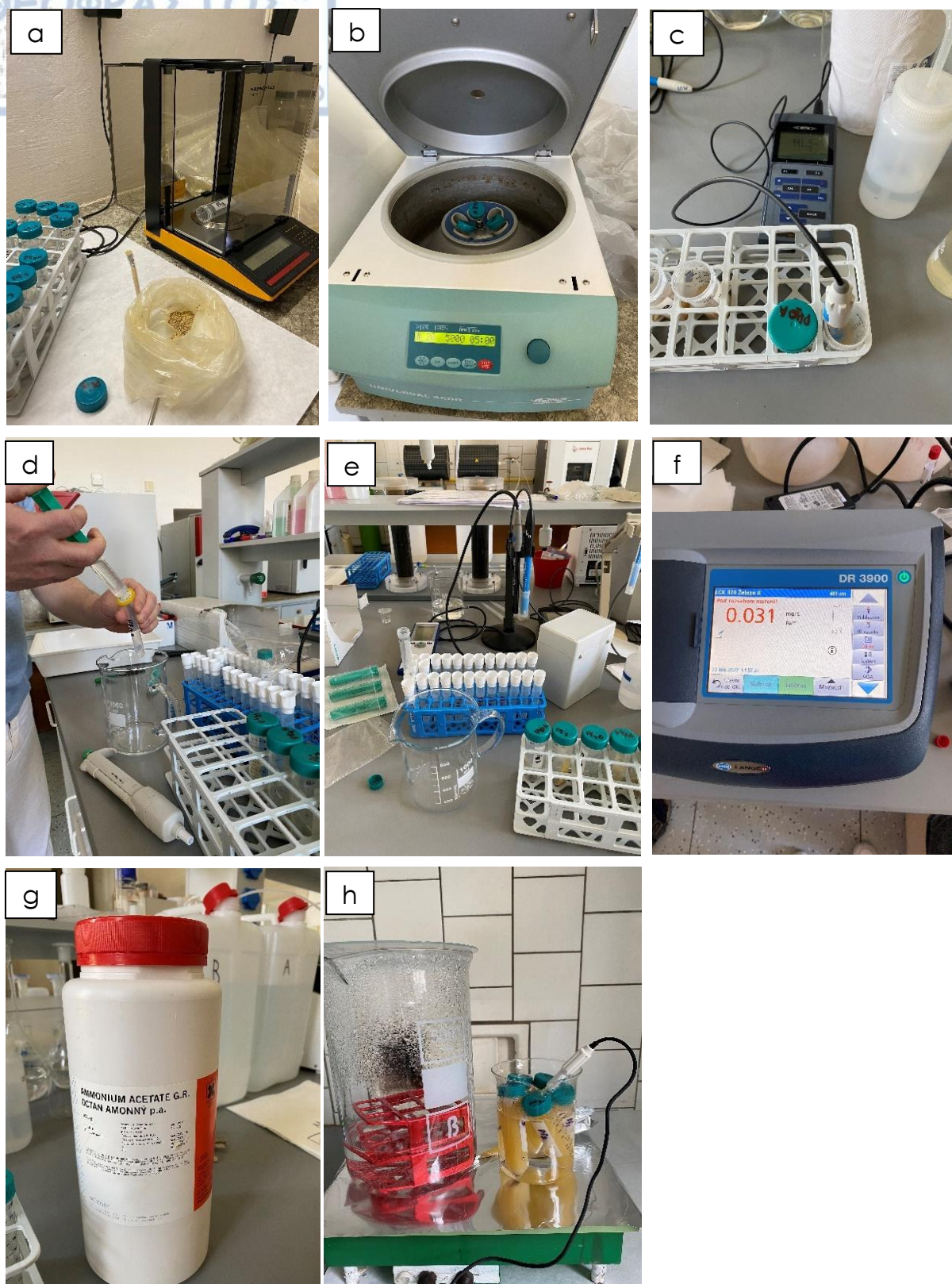
Fig. 11. Equipment used at the SE procedures: a. weight scale of the samples, b. benchtop centrifuge (UNIVERSAL 320R, Hettich), c. WTW multimeter and redox electrode for Eh measurement, d. processing of the samples after the centrifugation, e. 10mL testing tubes for \text{Fe}^{2+} and \text{Fe}^{3+} determination, f. DR 3900 spectrophotometer for the determination of \text{Fe}^{2+} and \text{Fe}^{3+} species, g. \text{NH}_4 -acetate used for the F2 fraction, h. heating of the samples at 80^\circ\text{C} for the F4 fraction.
