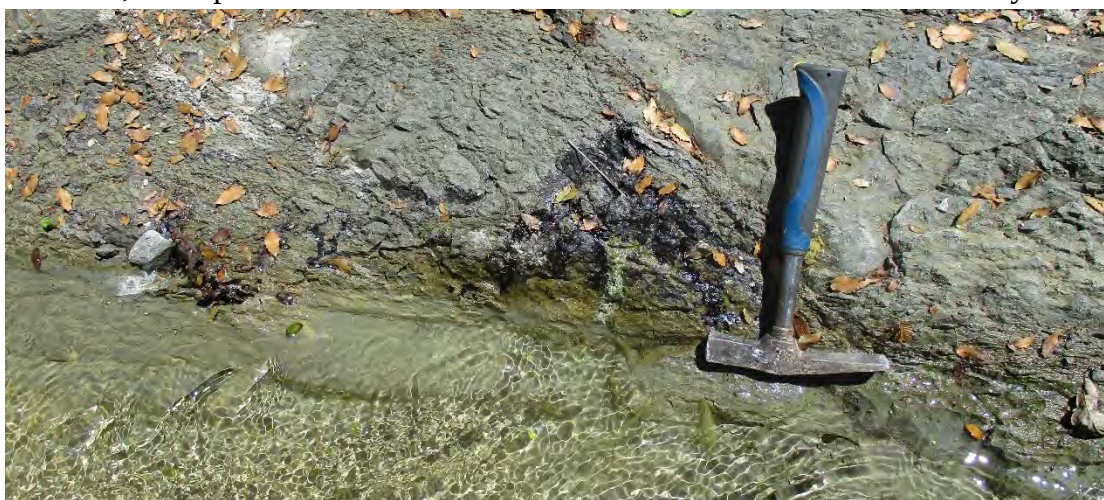
Figure 5. Solid bitumen (asphalt) seepage from fractured Miocene clastics (flyschoid) in the area of Dragopssa
