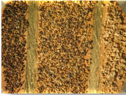
Figure 5: Sample C3 grain size 2.5 \Phi separated by sedimentation method in three parts ( \times 0.65 ).
