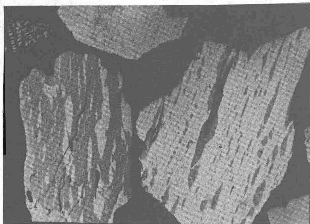
Fig. 3. Ilmenite (grey) with hematite (white) exsolution bodies of first and second generation (left grain). Hematite (white) with ilmenite (grey) exsolution bodies in two generations. Polished section, -N, oil immersion, X300
