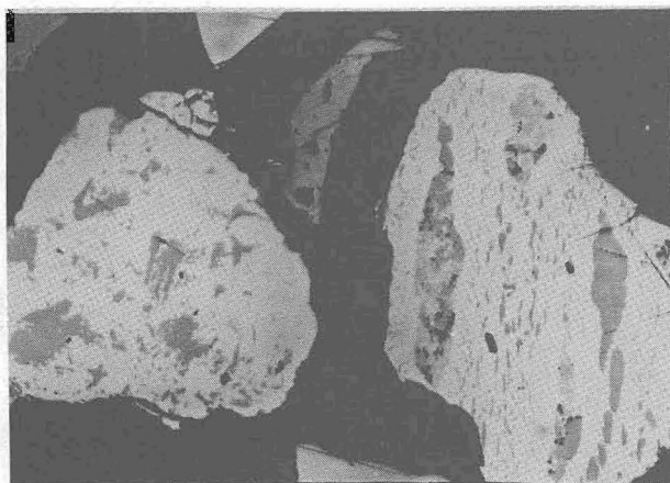
Fig. 4. Myrmekitic intergrowth of hematite (white) and ilmenite (grey). Ilmenite exsolution bodies within hematite in two generations (right grain). Spotty portions on ilmenite bodies are extremely fine hematite + rutile. Polished section, -N, oil immersion, X300
