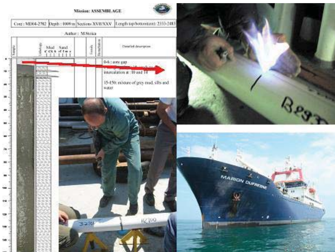
Fig. 5. Description of core (core: MD04-2782, depth 1009 m) on board of the French R/V Marion Dufresne. Setting methane gas from gas hydrates on fire (Dimitrov, 2010).
