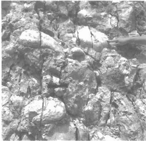
Figure 4: Pleistocene conglomerates in Kechries peninsula, affected by closely spaced joints
