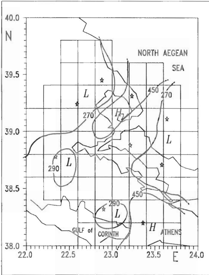
Fig. 4: Spatial distribution of  $Q_c$  at 2 Hz and for  $1.5t_1$  to  $1.5t_1+10s$  time window
