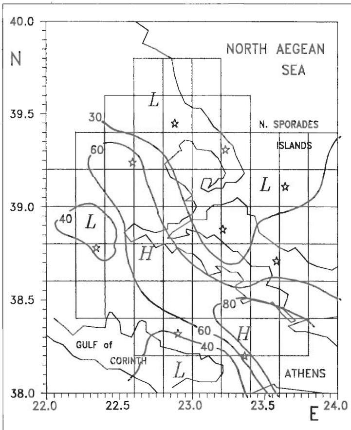
Fig. 3: Spatial distribution of  $Q_c$  at 2 Hz and for  $1.5t_s$  to  $1.5t_s+10s$  time window.
