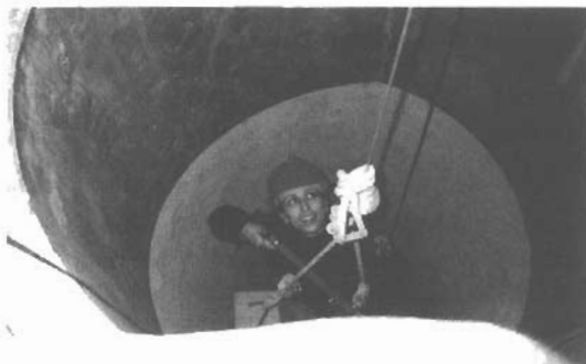
Figure 6. The operator at the top of the pyroclastic material ready to start GPR measurements another 8m downwards.
