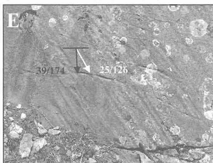
Figure 5 - (A) Panoramic view of Touthoa (TFZ) and Aetorrahi (AFZ) fault zones from northwest. (B) Fault surface of TFZ trending E-W with (D) two sets set of striations. (C) Curved low angle fault surface of AFZ with (E) a set of striations
