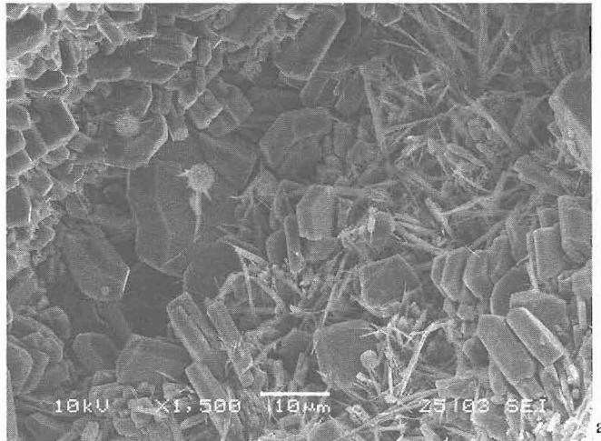
Figure 3a - SEM images tuff samples from Pâglişa area (located close to the studied area, for comparison). - Euhedral clinoptilolite crystals with minor opal-CT lepispheres and fibrous zeolite (mordenite?)
