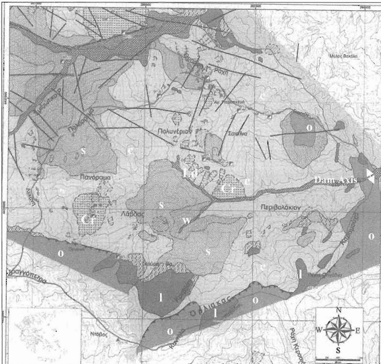
Figure 1 - Geological map of the Potamouli catchment area. Symbols are as follows: Chaotic flysch unit (c), sandstone unit (s), limestones (l), ophiolite unit (o), weathered mantle (w), creeping (Cr), landslide (Ld)
