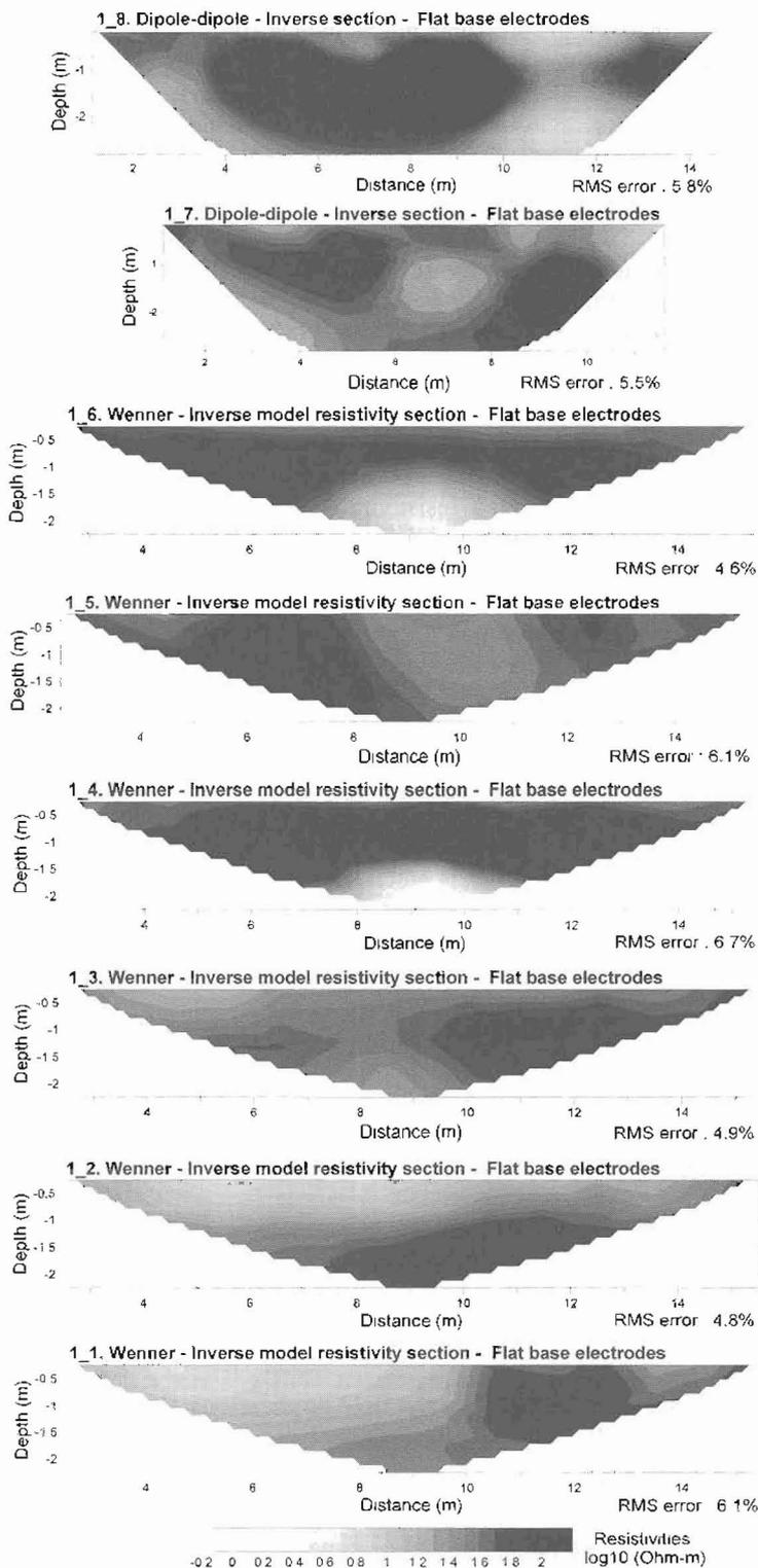
Figure 6 - Geoelectrical inverse model resistivity sections obtained by dipole-dipole and Wenner arrays. These sections have a northwest-southeast direction
