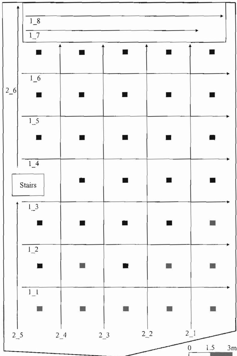
**Figure 4 - Sketch of the surveying area, in which the measured sections are shown. (1\_1) to (1\_8) sections refer to ERT's with northeast-southwest direction, while (2\_1) to (2\_6) sections refer to ERT's with northwest-southeast direction**
