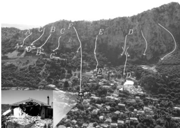
Fig. 5: Locations of the analysed Rockfall traverses. The location of a house destroyed by the rockfall is also shown.
