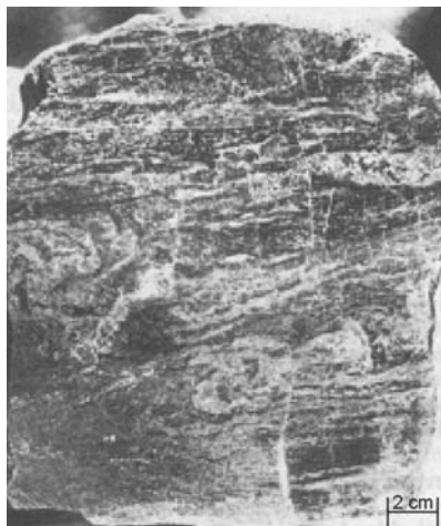
Fig. 3: Ore-bearing horizon made up of garnet, epidotes, quartz. The sulfides are finely disseminated in the rock. Crystallization broadly synchronous with the microfolds is visible; S. Gabriele, Funtana Raminosa Mine.
