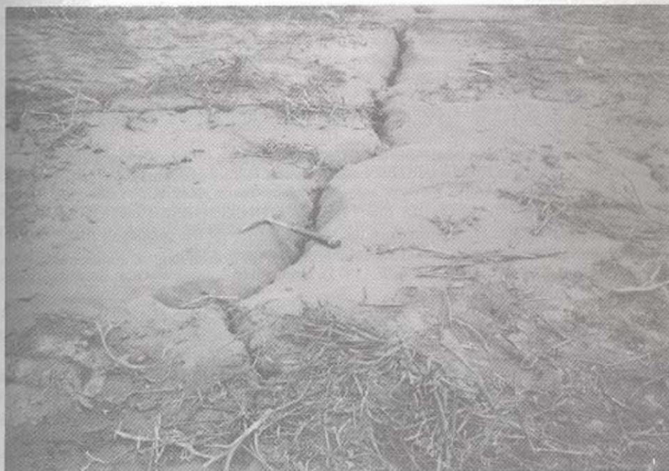
Fig. 9: Liquefaction in soil observed near the coastal position Bouka at ~ 6.5 km southeasterly from the village of Vartholomio, Elia.
