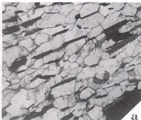
Fig. 5: Annealed textures in a quartzofeldspathic part of: a) a mesosome (x30, N-) and b) a cordierite aplite (x44, N+).
