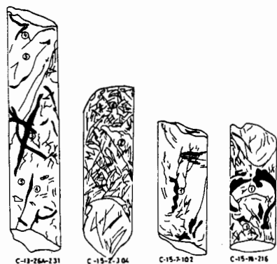
Fig. 3: Borehole cores, scale 1 : 1.1 - calcite; 2 - fissures; 3 - ferrodolomite; 4 - quartz; 5 - sodium metasomatites; 6 - fine veins (0.5 mm) - quartz, chlorite, hematite, carbonates, albite; 7 - hematite.
