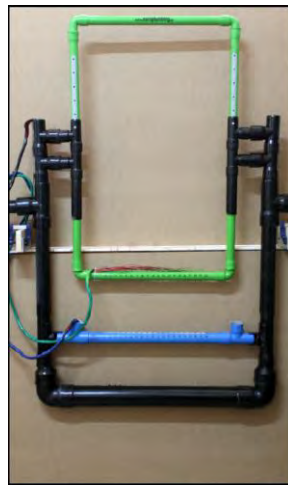
Figure 5 – Construction used for the experiments. It consists of three parts (green, blue and black) which distance can be chosen by will. Whole construction is made by plastic parts for conductivity reasons.
