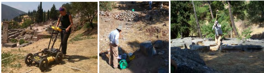
Figure 2 - Details of the geophysical methods with GPR (left), ERT (center) and SRT (right) that were applied in the area A of the site.
