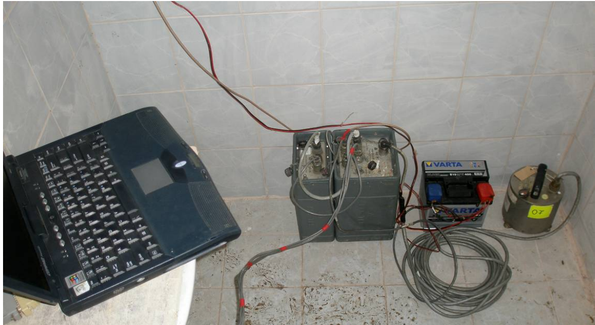
Figure (4.2) Picture of the installation of the seismological station with codename ANAN. It is illustrated from right to left, the seismometer, the battery, the digitizer, the disk storage of data and the computer (after Tsapanos et al., 2011).
